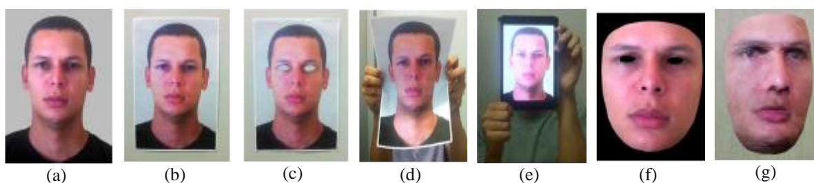
Figure 2. Types of presentation attacks (a) valid user, (b) printed flat photo, (c) eye cut photo, (d) warped photo, (e) video playback, (f) synthetic mask, and (g) paper cut mask [9]
